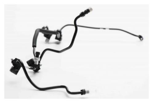
Made from thermoplastic material, our high-pressure liquid line is designed for the air conditioning line and connects the compressor to the evaporator. Its benefits for our customers: lightweight design and high flexibility.
