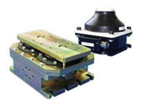
Our active noise and vibrations control system STRACTIVE<sup>T</sup> cancels incoming vibrations by generating a dynamic force of the same magnitude in opposite phase through the use of electrodynamic actuators. It improves vibration insulation in the range of 10 to 1.000 Hz (-12 to -36 db).
