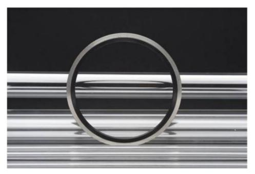
The bonded seal consists of a metallic insert with a vulcanized rubber compound profile which is bonded to the internal diameter.
