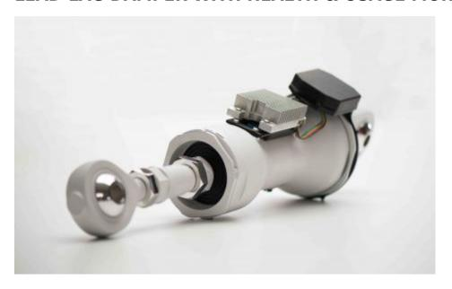
With our Embedded Health and Usuage Monitoring System, sensors mounted on frequency adaptors for helicopters monitor displacement, force, pressure and temperature. Data are analyzed and stored in flight, allowing the component's health to be assessed and data on real operating conditions to be saved.
