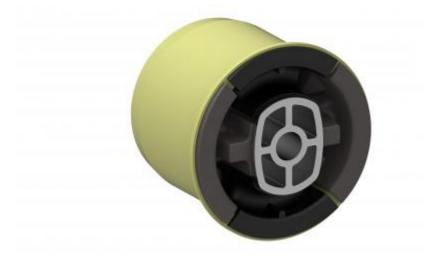
Our Dual Compound Bush is a solution for the rear axle twist beam. Thanks to the stiff rubber used in the horizontal axis and the low dynamic stiffness in the vertical axis, it enhances passenger comfort. It offers a performance between conventional and hydrobush solutions. It is designed to dampen vibrations from the road and absorb shocks. It plays a key role in improving vehicle performance, safety and passenger comfort.
