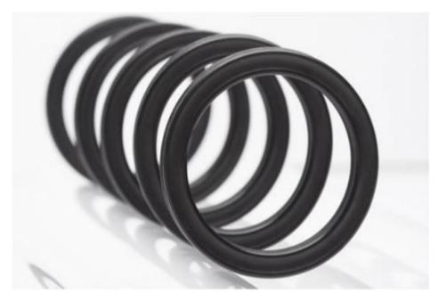
X-Ring has a cross-section with 4 lobes offering a double sealing line. Just like for O-Rings, there is no direction of assembly.
