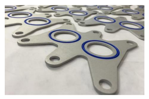
This specific seal design allows separating static sealing and tightening functions. It makes it easy for assembling, more robust, and increases its life duration. The choice of compounds and substrates enables it to operate in extreme conditions without compromising on weight. Our plate seal is qualified for industrial, aerospace and military applications.
